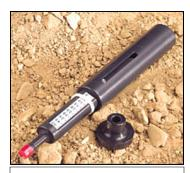
A penetrometer is an excellent tool to use for a manual test. It will give you the unconfined compressive strength of the soil which can be used to properly classify the soil. They are less subjective than the other manual tests. Approximate cost \$60
